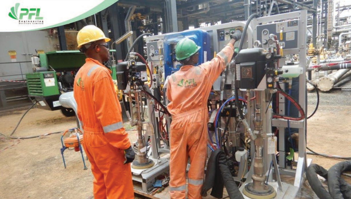
Graco XMPlural Component Sprayer for Passive Fire Protection (PFP)
