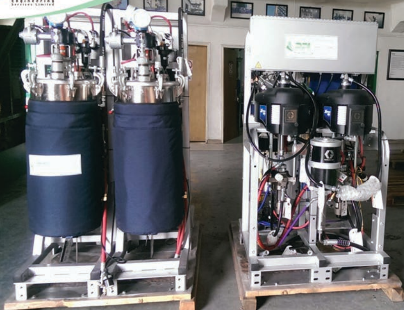
Graco XMPlural Component Sprayer for Passive Fire Protection (PFP)
