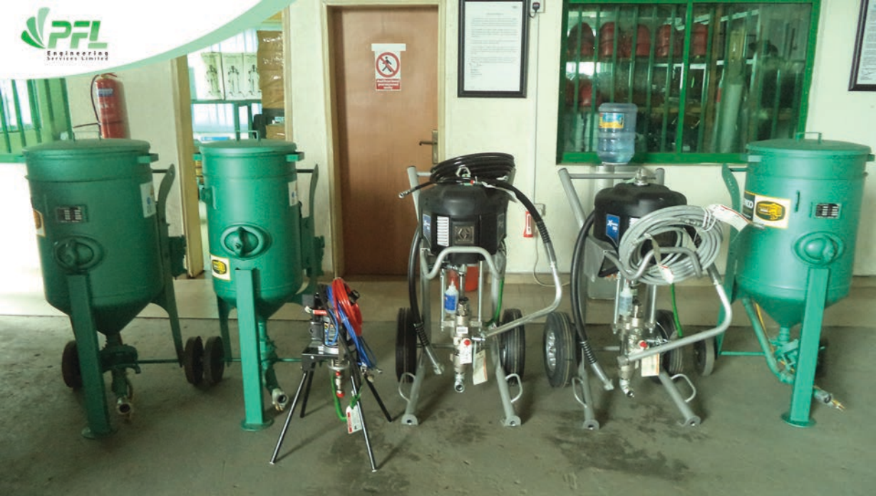
Blast Pots for Blasting and Painting
